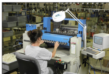
Automatic winding of bobbin-wound coils
